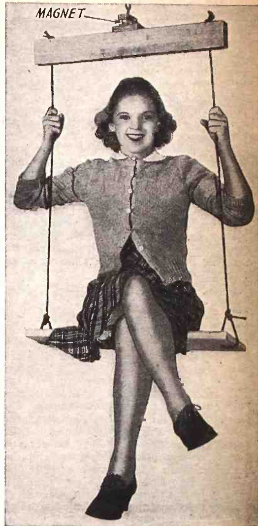
Courtesy General Electric Co. A small Alnico magnet upholds girl and swing.
