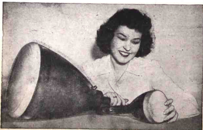
At left is one of the large direct-viewing cathode-ray tubes. At right, the much smaller high-voltage projection-type tube described above, which is employed in the RCA large-screen equipment.
